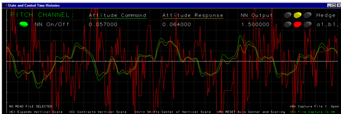
Figure 7. Pitch Channel Flight Test Time History for Combined Pilot and Square Wave Input using the Error Observer Approach with PD controller. Design natural frequency is 8.0 radians per second with hedge actuator model time constant reduced from 0.04 to 0.01.
